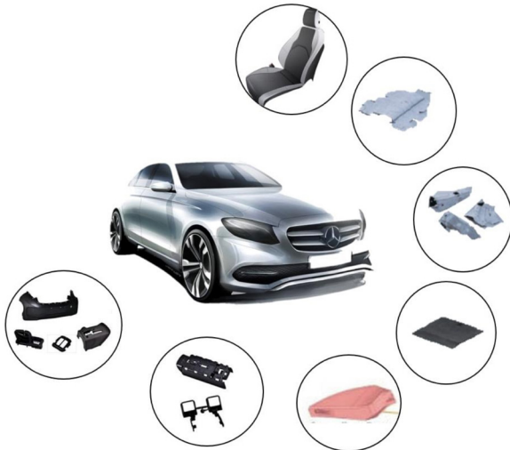
Fig. 3. Components of Mercedes E-Class produced by using natural fiber composites.
