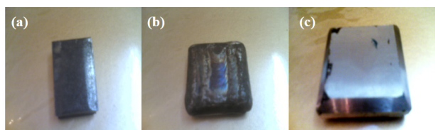
Fig. 1. The images of a plate; (a) primary plate (before creptation), (b) plate after creptation, and (c) polished crept sample.
